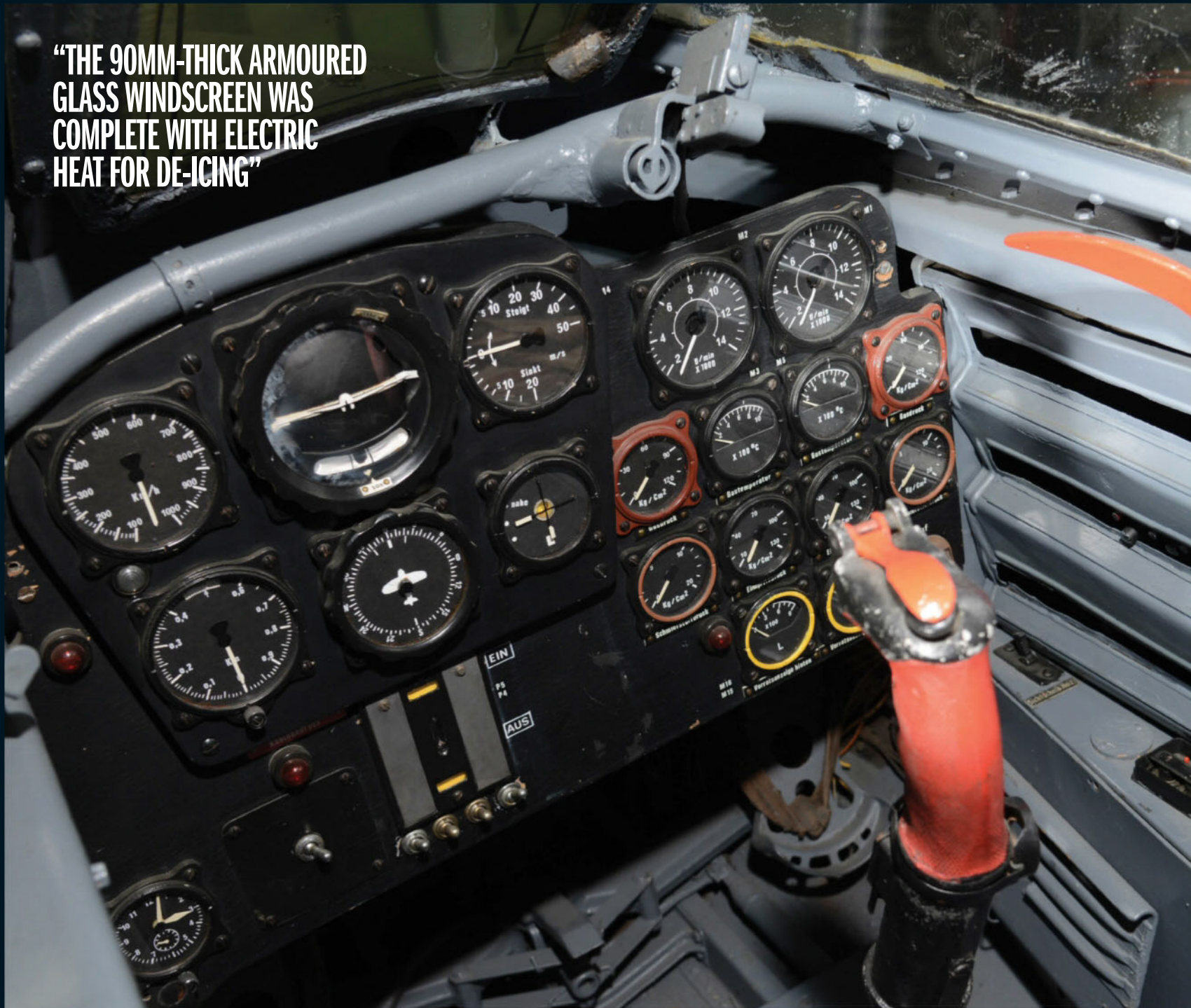
The main instrument panel of the Me 262 cockpit allowed the pilot to view flight characteristics, gauges and armament controls
